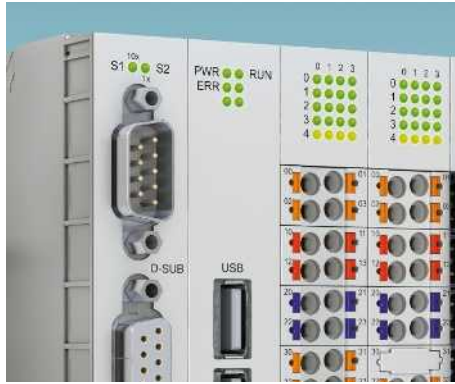
Fig. 35: Light guides in the ME-IO housing for a compact indicator area
