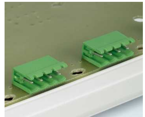
Fig. 24: Edge assembly on a profile housing
