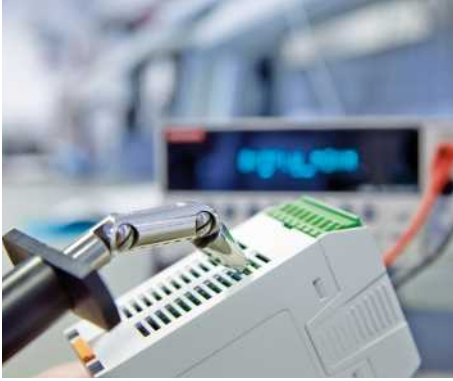
Fig. 65: Test for mechanical seal tightness
