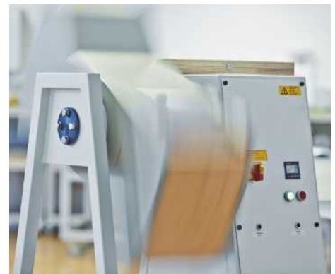
Fig. 64: Tumbling barrel test
