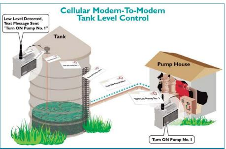
Cellular modem-to-modem text message communications can be used for autonomous tank-level control
