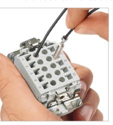
Looking closer at each of these termination methods, let's start with crimp contacts. Crimp contacts are great for large-volume production, especially when available in reeled form to facilitate automated crimping, though it is possible to automate the crimping of machine-turned contacts as well. Stamped-andformed contacts (or punchrolled) are easily provided on reels, and often accept a range of wire sizes. Ma-
