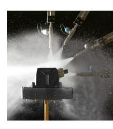
these tests do not address spray water, a dual IP rating is usually applied. For example, if you see something with IP66 and IP67 ratings, you will know that both of those spray and submersion conditions have cleared testing successfully.
