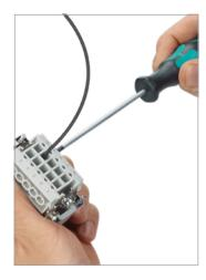
Next on the list is screw terminations, whose popularity cannot be denied. These terminations don't involve the need for any special tooling, and the preinstalled contacts accept the widest range of wire sizes. While it is recommended that wires be ferruled and that the screws be tightened to the manufacturer's recommendations using a torque driver set, reality tells us
