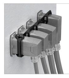
single-latched connectors would be best stacked end-toend, while dual-latched connectors are best stacked sideto-side to allow free access to the latches themselves.
