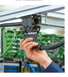
While the environmental conditions are a huge part of the considerations, there are still several other points to evaluate. Understanding the location of the connection and the physical limitations that the surroundings impose on the connector will be important. If the connector is attached to a panel or cabinet wall, a panel mounting base will be in order. If this is part of a distribution network outside of an enclosure, a
