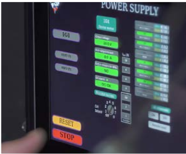
Figure 4a and 4b: Phoenix Contact's TRIO power supply with integrated circuit breakers ensures reliability. If a breaker trips, the technician can easily reset it from an HMI screen without opening the enclosure.
