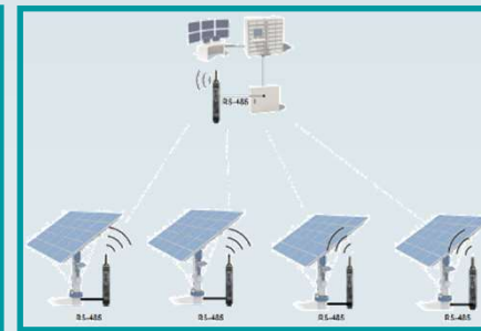
Wireless monitoring of tracking systems
