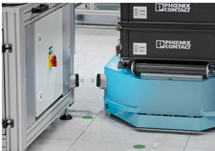
Figure 3: Data is transmitted across an air gap over a distance of up to 100 millimeters and is insensitive to the existing sources of WLAN interference.
