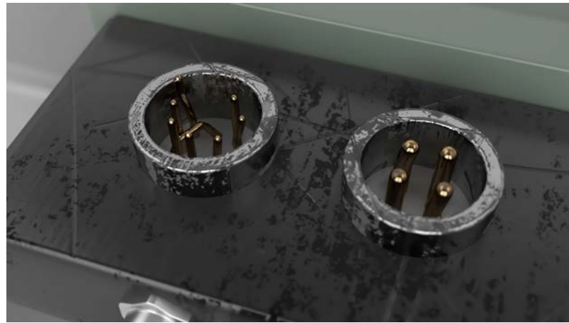
Figure 5: If connectors are frequently disconnected and plugged in, the contacts can become dirty and bent. This leads to unplanned or unforeseeable production stoppages and frequent maintenance intervals.
