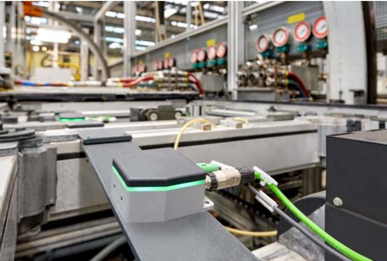
Figure 4: A NearFi coupler for contactless communication is located at each processing station and on each workpiece carrier.
