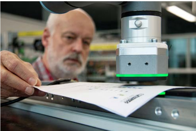
Figure 2: NearFi enables power and data transmission, even through non-metallic materials.
