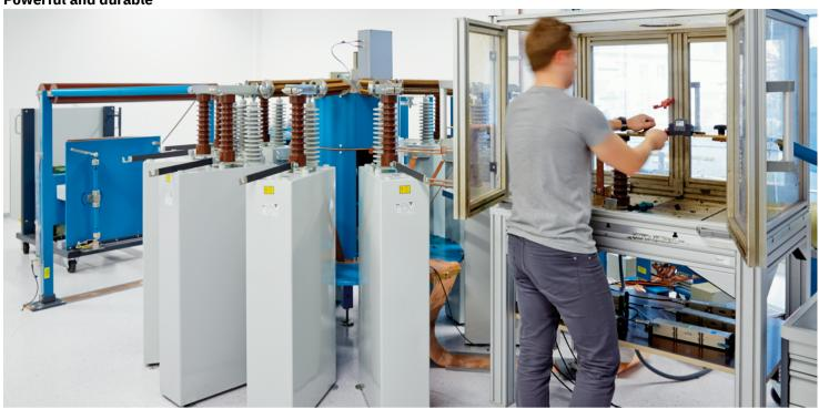
The surge protective devices are subjected to a large number of tests and examinations during their development phase in the in-house, certified pulse and high-current laboratory.
