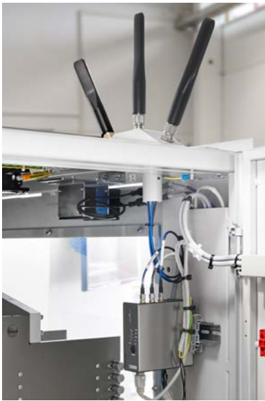
Figure 4: Before the Access Point WLAN 2100, the WLAN 5100 with external antennas was used in the first years after market launch.
