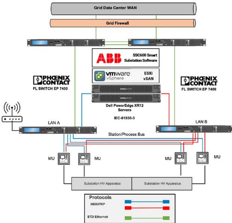
**Figure 1.** Physical Architecture of vPAC Platform
