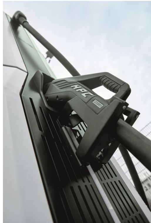
Figure 4 - High Power Charging connector from Phoenix Contact: electric vehicles are easily charged in just a few minutes
