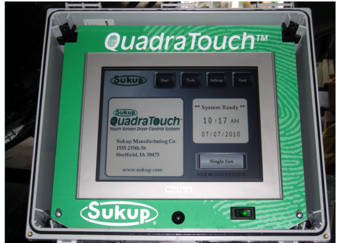
The QuadraTouch control system HMI can be located up to 200 feet from the dryer. It connects to the PLC, which is located in the power box on the grain dryer, via Ethernet.
