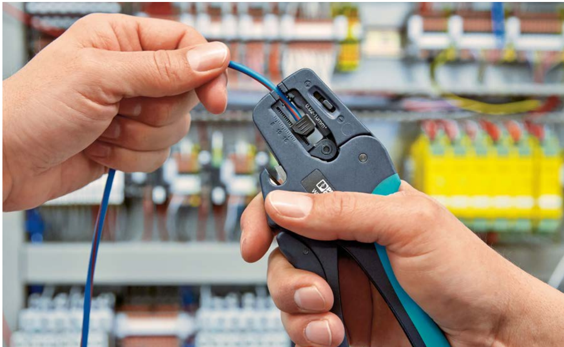
Figure 3: The automatically adjusting stripping pliers are the recommended hand tool. These make stripping different conductors simple and reliable.
