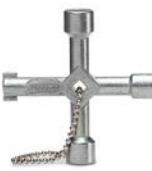
Universal control cabinet key with strong chain and snap hook for nine closures: 5, 6, 7 - 8, 9 - 10 mm square, 7, 8 - 9, 10 - 11 mm triangle, 3 - 5 mm two-way key bit, 6 mm semicircle
