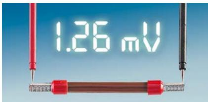
The voltage drop must not exceed 3.2 mV before or after the test, nor may it exceed 1.5 times the value measured at the start of the test.
