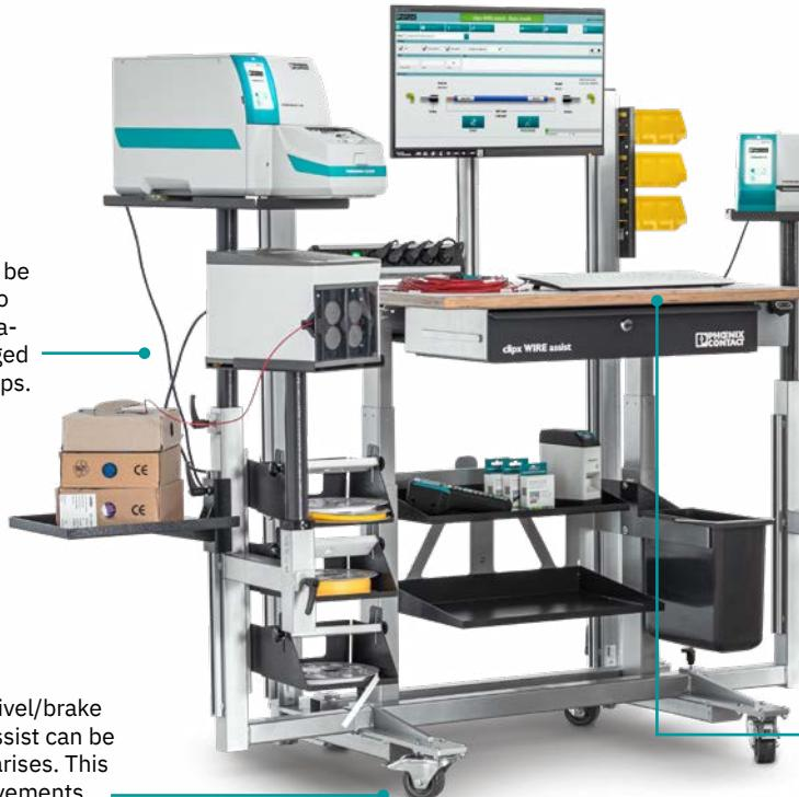
Equipped with special swivel/brake casters, the clipx WIRE assist can be used wherever the need arises. This reduces unnecessary movements and saves time.
