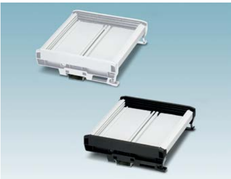
Housings made of PVC (UM-BASIC) or PA (UM-PRO) for application temperatures up to +50°C or up to +100°C
