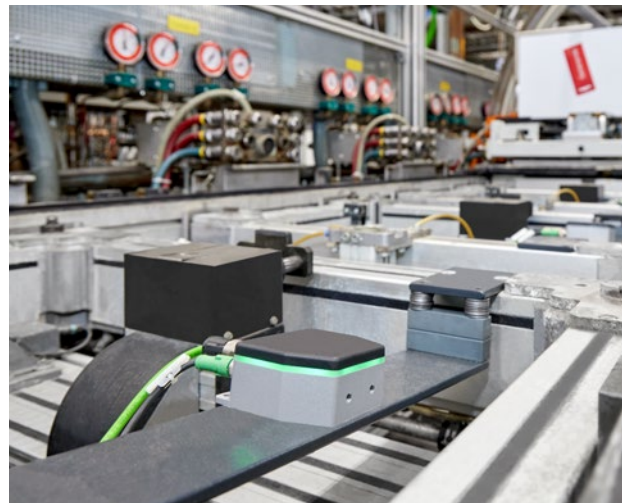
A NearFi coupler for contactless data transmission is installed on each workpiece carrier
