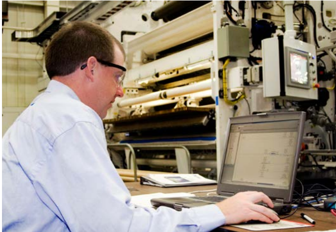
Figure 3: With a Phoenix Contact wireless radio installed in the machine, an operator can use a tablet or laptop to control the machine from any nearby location.
