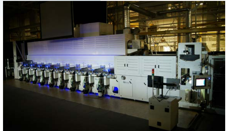
Figure 1: Phoenix Contact communications make it possible for a local operator to control this Aquaflex web printer from a handheld device, and for engineers at PCMC to access the automation system remotely.
