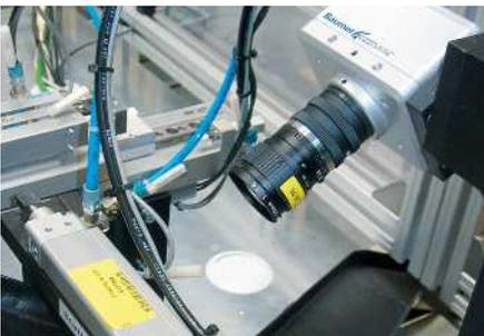
Quality inspection using optical camera systems
