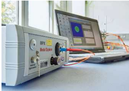
Prevention of attenuations and reflections through end-face testing in fiber-optic cables
