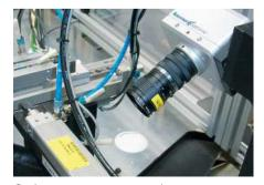
Quality inspection using optical camera systems
