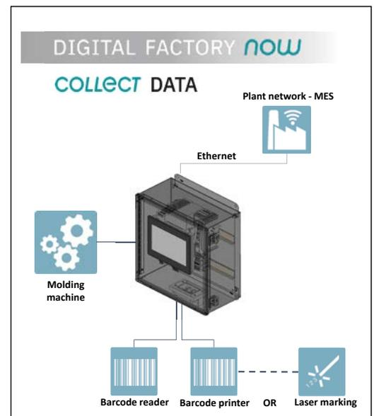
Simple configuration for interfaces results in faster development. The system is easy to expand, so it is future-proof. Formatting of data for MES increased connectivity. The built-in cybersecurity for OT to IT ensures efficient utilization of resources. The HMI has a built-in interface for local or mobile use.
