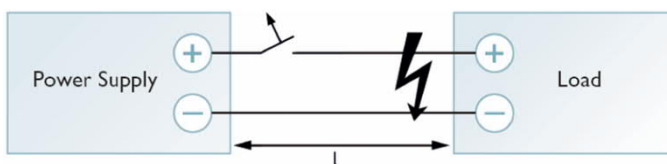
Schematic diagram of the maximum cable length
