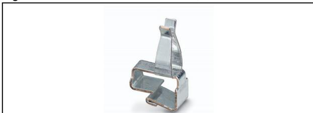
When you snap the housing onto a DIN rail, you can establish a conductive connection between the PCB and DIN rail. The functional ground contact (FE) does not satisfy the demands on a protective grounding connection (PE).
