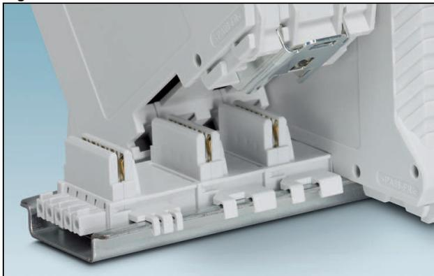
The ME...TBUS DIN rail connector is integrated into the DIN rail. The bus connector has 5 positions for energy supply and data transmission. It connects several electronics modules, which are mounted on the DIN rail. When you remove a device from the topology, the contact chain (in the case of parallel contacts) is not interrupted.
