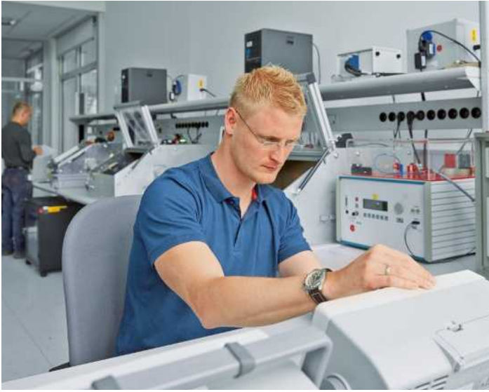
Fig. 26: Fully automated testing system for determining the overload and failure behavior of surge protective devices in accordance with IEC 61643-11 [6]
