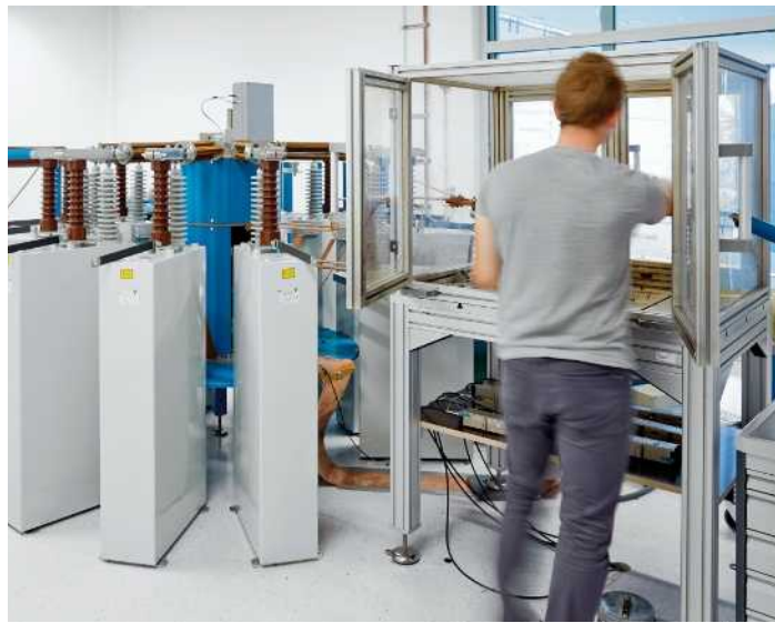
Fig. 27: Lightning surge current generator
