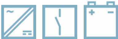
Power supply UPS module Energy storage
