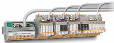
Another hidden benefit of moving the relays to the cabinet in a system cabling solution is that a user can mix and match different relays on a per-channel basis. For example, Relay 1 can be an electromechanical relay, while Relay 2 can be solid-state, and Relay 3 can be double-pole double-throw, etc. This allows for much greater flexibility in an application compared to the uniform nature of all identical relays in a relay output card.
