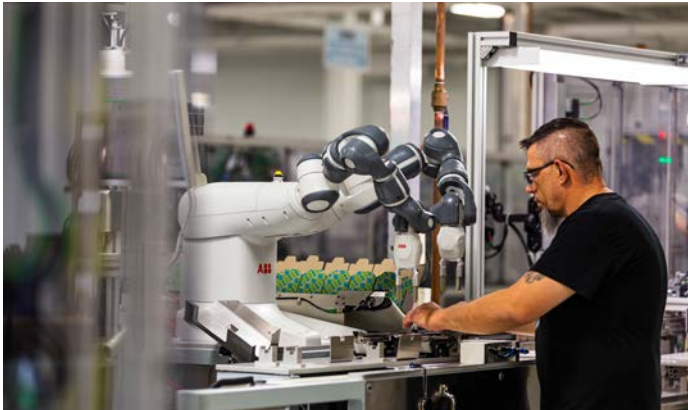
Figure 2: Frank Sabatini, lead production operator in the DC Automated Assembly department, performs a changeover, setting up the cobot to run a different part.
