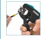
A subgroup of self-adjusting crimping pliers is equipped with a rotating die. The conductor can be inserted from the front or the side. This enables conductors to be crimped conveniently, even in confined work areas.
