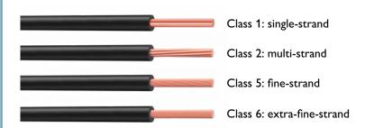
Ferrules in accordance with DIN 46228 part 1, 4, and UL 486F-A, E, F are designed to accommodate class 2, 5, and 6 conductors. Class 1 conductors, also called rigid conductors, are generally not crimped with ferrules. NOTE: Aluminum conductors may not be crimped with copper ferrules!
