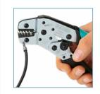
This widely used and universal type of crimping pliers is based on the scissors principle and is available with dies for different types of contact. With these tools, each cross-section has its own die cavity or nest, requiring close attention to correct positioning.
