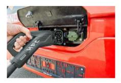
Outside of the vehicle, the charging process is completed using a separate Ebusco charging station. The electric bus manufacturer produces charging stations that are specifically designed to handle the demands of heavy battery packs. Phoenix Contact charging cables and power electronics can also be found within these charging station systems. This ensures an optimal charging process throughout the overall system.
