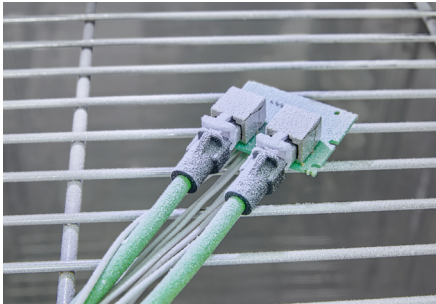
Durability test under extreme climatic conditions
