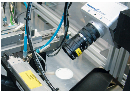
Quality inspection using optical camera systems
