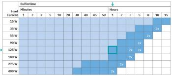
2x: In this case, two battery modules of the same capacity are required. The data is based on an ambient temperature of +25 °C at start of use.
