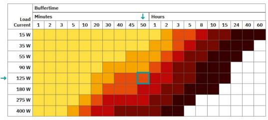
The data is based on an ambient temperature of +25°C at start of use.
