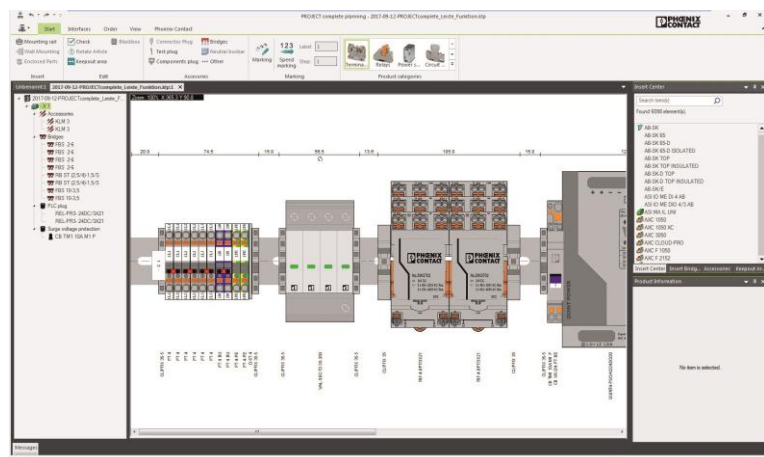
Figure 2 - Convenient interfaces to the CAE system: terminal strips and markings are created with a high degree of automation
