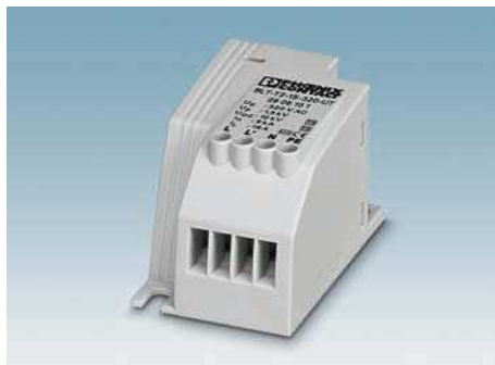
Type 2 surge protective device BLOCKTRAB for insulation class I with PE connection for direct use in the lamp or in the cable junction box.
