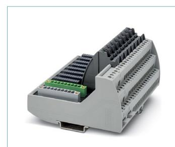
IOA-compatible, 8-channel base interface module with two rows of screw terminals for direct connection to I/O card. Each individual channel has four connections (A, B, C, D) and multiple shield options.
