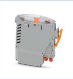
A single input/output accessory (IOA) is inserted into each channel of the VIP-ER base module. In turn, a total of 32 IOAs are required for a single Honeywell 32-channel Universal I/O IOTA. Simply insert each IOA into the IOA guide found on each VIP-ER base module. A variety of IOA functions are available and should be selected based on the configured signal type.
