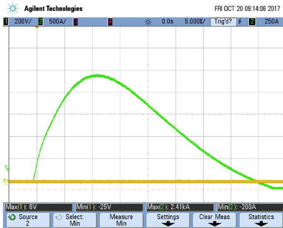
$I_K (8/20\mu s) 2,4 \text{ kA} @ U_{OC} = 6 \text{ kV}$
