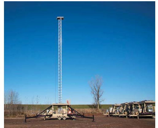
Figure 1: The PTX-100 tower is a robust and stable mobile tower. It can stand up to hurricane-level wind speeds without the need for ground-penetrating guy wires.
