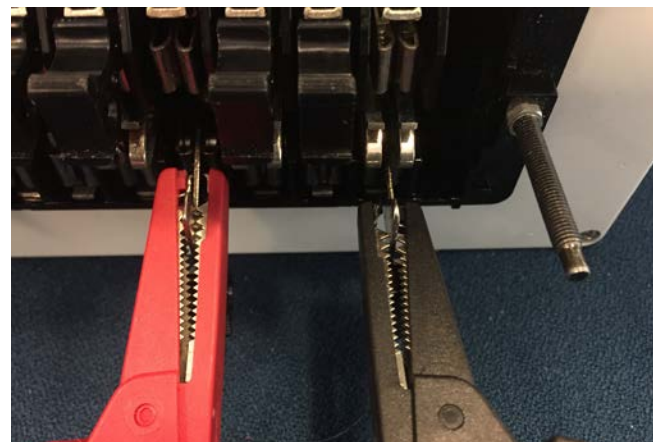
Figure 4: Voltage measurement using alligator clips.
