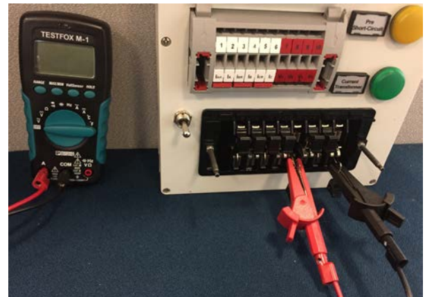
Figure 7: Alligator clips used to take voltage readings.
