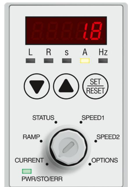
Operator interface of the speed starter
