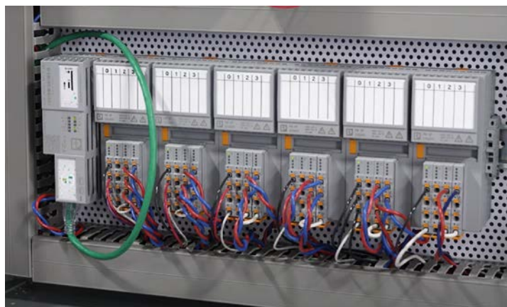
Figure 3: More complex machines will require a PLC to collect and process data. Rather than just gathering the data, the PLC can preprocess the data with scalars, multipliers, and more. An open control system like PLCnext Technology can then send the data to an internal server or external cloud service, such as Amazon Web Services (AWS) or Microsoft Azure, for further use.
