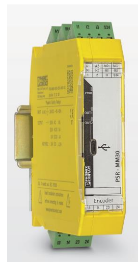
Figure 1 - The PSR-MM30 can monitor up to three different speed thresholds on one machine, along with zero-speed monitoring
