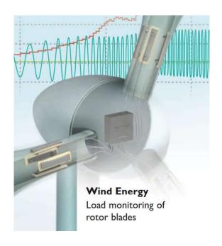
The rotor blades are subject to large dynamic forces which can lead to structural damages over the service life of the blades. Damages can be recognized early by continuously monitoring loads and vibrations. These data allow a perfect load-based regulation of the wind power plant, thereby reducing the stress on the blades to a minimum.
