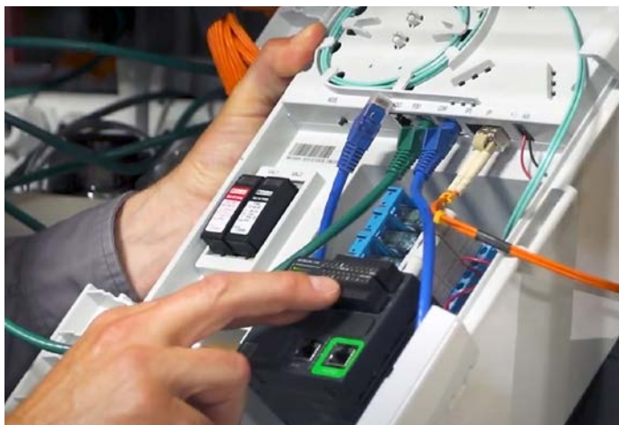
Figure 3: The Smart Ethernet Box is an outdoor PoE switch with integrated power supply, surge protection, splice tray for fiber optics, and a DIN rail for additional accessories.
