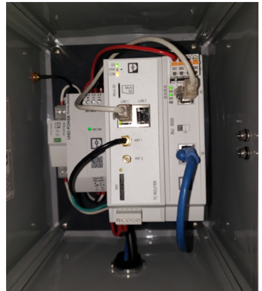
Figure 2: Phoenix Contact's TC Router, an industrial 4G LTE mobile router that enables high-speed Internet connectivity via mobile networks.
