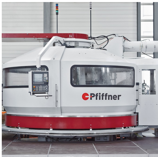
Rotary transfer machine from Pfiffner for mass production of precision parts
