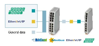
The new unmanaged switch series features enhanced data traffic prioritization for automation protocols. The real-time properties of PROFINET and EtherNet/IP™ automation networks are thus supported. This results in more stable networks and increased system availability.
