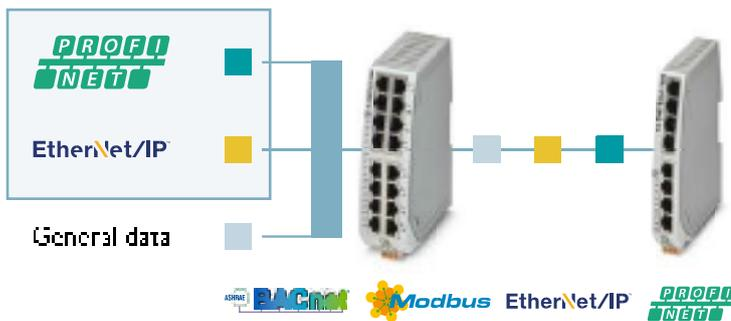
The new unmanaged switch series features enhanced data traffic prioritization for automation protocols. The real-time properties of PROFINET and EtherNet/IP™ automation networks are thus supported. This results in more stable networks and increased system availability.
