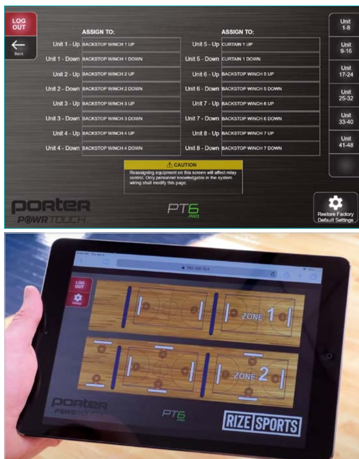
Figures 3A and 3B: The custom HMI makes it easy for rec center staff to control up to 64 pieces of equipment.
