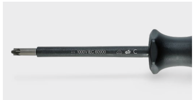
Marking on a VDE tool: The letter "C" indicates that it may be used at low temperatures
