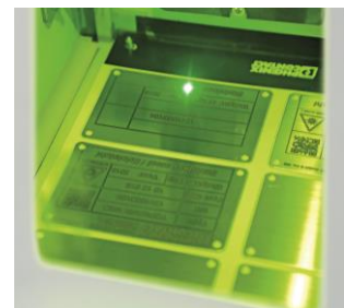
Figure 2 - As resilient as the material itself: The material - in this case high quality stainless steel - is marked using laser technology by removing the material
