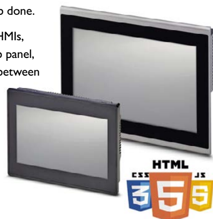
Figure 3: HTML5 web no longer rely on specific communication protocols or PLC models, so they blur the line between HMI's and IPC's even more.
