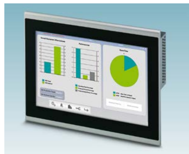
Figure 2: If your HMI has a capacitive-touch screen, you can use gesture control, like swiping or pinch-zooming.
