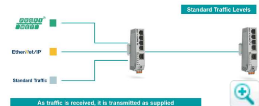
FL SWITCH 1000 Series Prioritization of Automation Protocols (IEEE 802.1Q)
