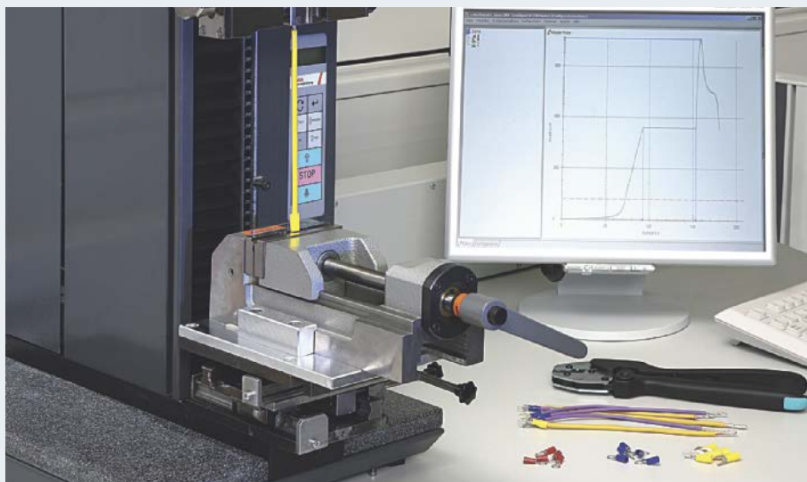
Conductor pull-out test
