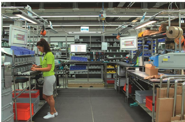
Figure 4 - Terminal strip production in full flow: a production system design based on the flow principle minimises lead times
