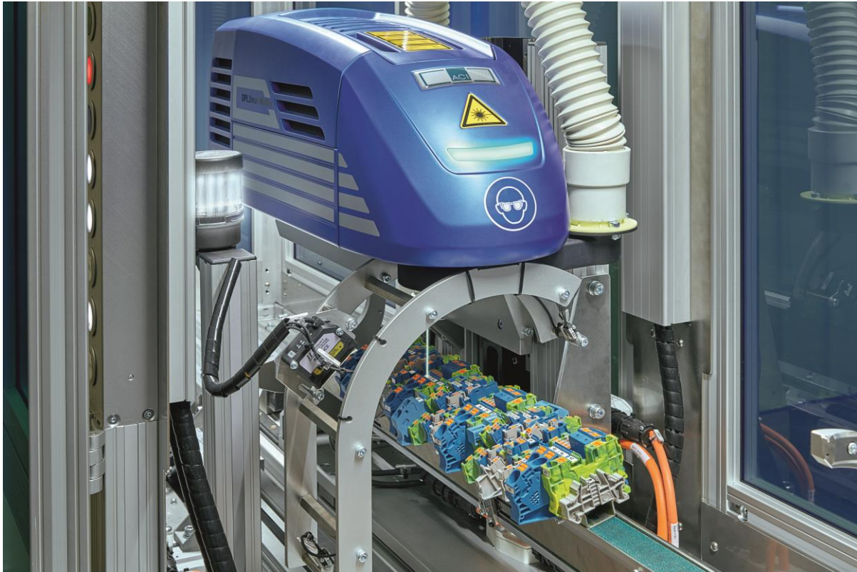
Figure 3 - Making its mark: laser marking of fully assembled terminal strips significantly reduces the amount of effort required for marking
